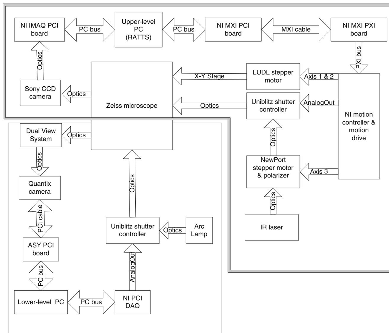
**Fig. 3** Hardware diagram of system to study sperm motility and energetics. The upper-level system includes the components in the *double-line box*, and the lower-level system includes the components in the *single-line box*
