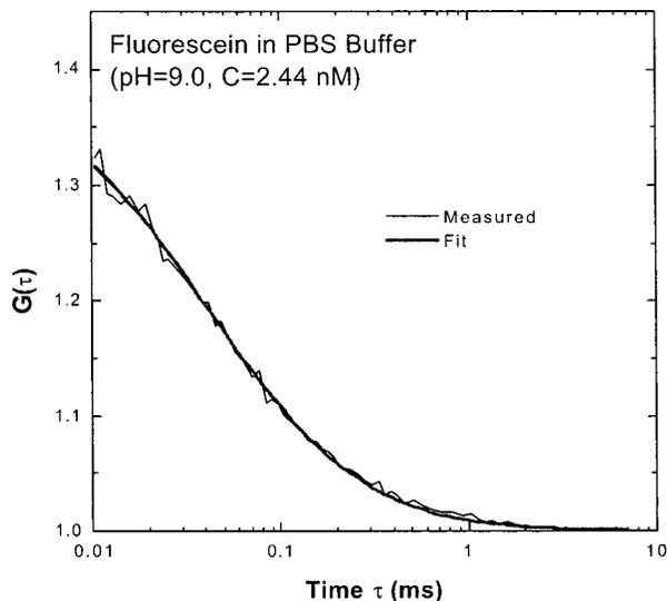
**Fig. 2** Autocorrelation curve  $G(\tau)$  of fluorescein dyes in PBS solution at concentration of 2.4 nM used for the calibration of our FCS system.
