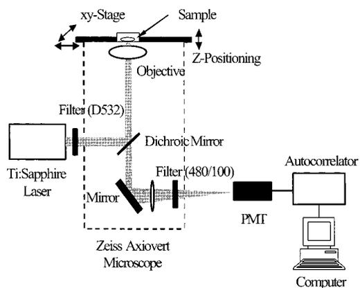
Fig. 1 Experimental setup for two-photon FCS measurements.
