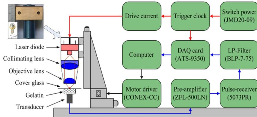
Figure 1. Schematic diagram of the VIS LD-OR-APM system; inset: the photo of the laser diode excitation.
