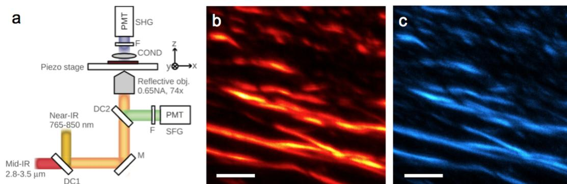
Fig. 1. Collinear SFG microscopy with a high-repetition rate light source. a) Layout of the SFG microscope. DC: dichroic mirror; M: reflecting mirror; F: bandpass filter. COND: condenser; PMT: photomultiplier tube. b) Epi-SFG image of collagen from hawk cornea at 2945  $\text{cm}^{-1}$  (CH stretch). c) Forward-SHG image of the same cornea sample. Scale bar is 20  $\mu\text{m}$ .
