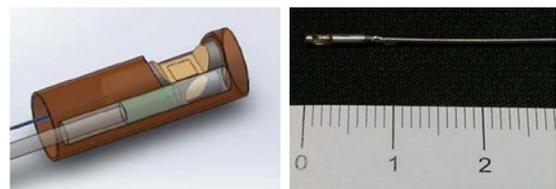
Fig. 2. Structure of the trimodality endoscopic probe: the optical probe and ultrasound transducer were placed side by side. The rigid portion of the probe is 0.7 cm and the diameter is 1.2 mm. The scale is in centimeters.
