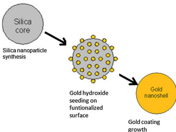
**FIGURE 2.** Synthesis of silica-gold nanoshells.
